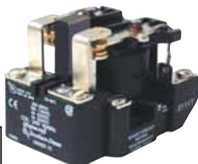
199B DPDT WITH MAGNETIC BLOWOUT FOR DC ARC QUENCHING
